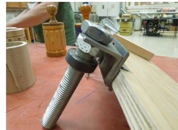
The three photos below show the index wheel pointer and mount. The pointer is bolted into the base, which sits on the lathe bed rails and held with magnets. The pointer height has a slight adjustment range depending on the index division set used. The wheel is not shown, but mounts on the spindle
