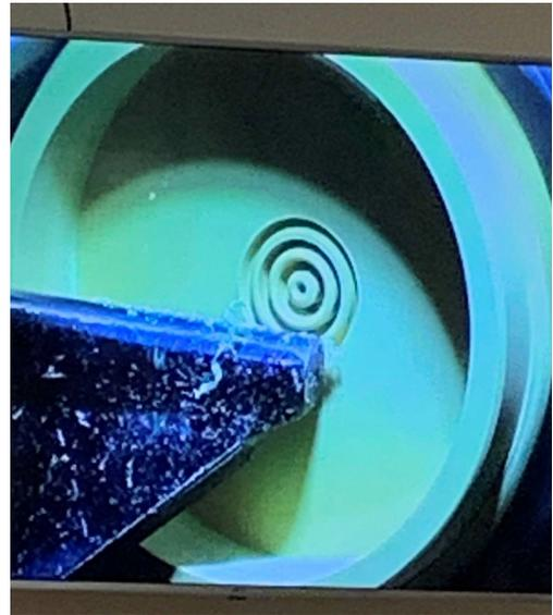
Above, after the grooves on the front face are completed, the part is removed from the chuck plate, flipped 180° and mounted in the chuck. Grooves are then added to rear of the part. The groove depth is made so that the bottom of the groove coincides with the plane of the grooves on the front side.
