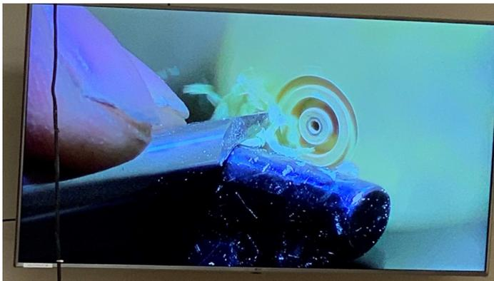
Above, the blank is mounted on the chuck insert using the two pins to register the blank position. The grooves are cut to the depth of the intersection plane between the work performed from the front and rear faces of the blank.
