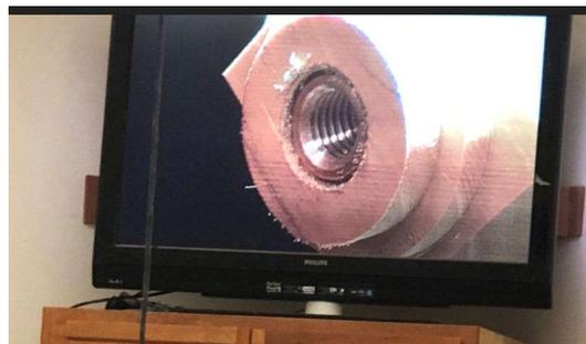
Handle blank drilled & insert installed
