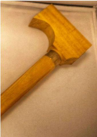
Handle blank assembled onto top section of shaft
