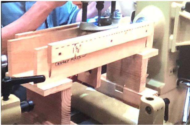
Setting the tapering jig onto lathe
